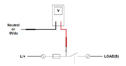
This method of determining the fuse / breaker status was chosen over a status LED because a blown fuse indicating LED would produce a leakage current and would only indicate when the relay contact was closed while a fuse healthy LED would require a neutral or OV terminal to be added to the module. Fuse status LED's also tend to be optimized for a particular voltage while the test point method means a single module is suitable for 24Vdc and 120Vac loads.
