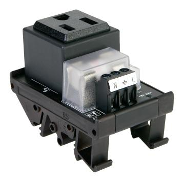
The latest addition to Emphatec's line of AC outlet modules is the ACFT version with on-board branch fuse. The fuse, a T-class type, provides a 10KA interrupting current rating. An LED provides indication that the fuse is healthy and the power is applied to the module.
