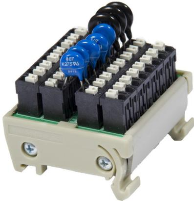
MOV's are often added to control circuits to provide overvoltage/transient protection. Since MOV's breakdown and eventually fail as a result of the transients they are eliminating they should be readily accessible for inspection (they often change colour, expand and sometimes explode with age/exposure to transients) and replacement.
