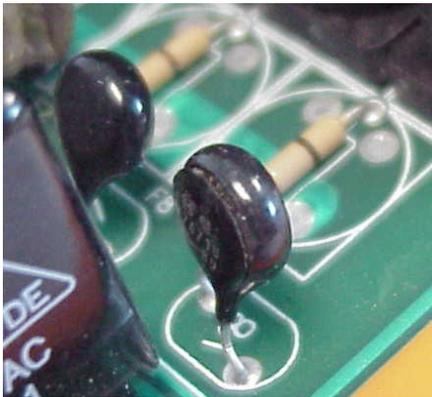
The photo to the left show's what happens to MOV's when they are exposed to repeated voltage transients. The body of the MOV expands and if the device is a lighter colour they also discolour.
